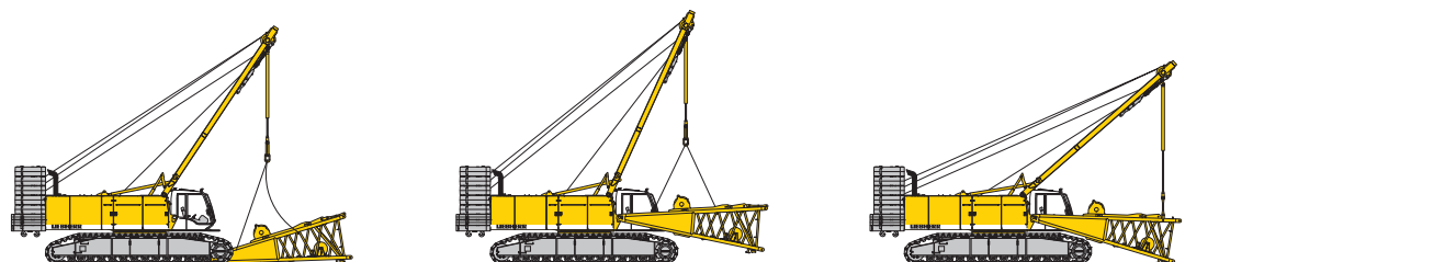
Unloading and assembly of boom foot
