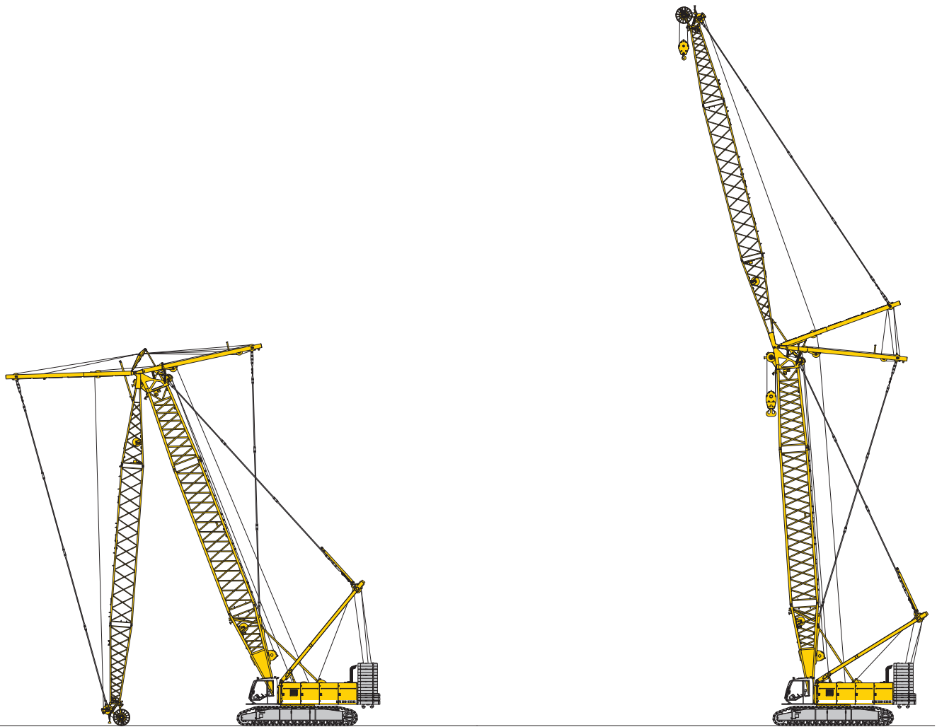
Erecting of main boom and luffing jib
