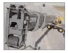
The 160 ft. (48.8 m) 5 section Full Power boom incorporates the "U" shaped MEGAFORM<sup>TM</sup> design, which eliminates stiffeners, thus reducing weight and increasing capacity.
