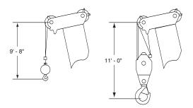
Dimensions are for largest Grove furnished Hook Block and Headache Ball, with Anti-Two Block Activated.
