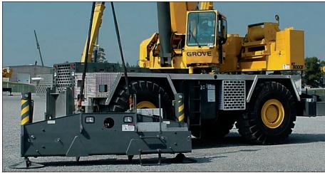
Removable front and rear outrigger boxes provide up to 19,374 lbs. (8 788 kg) of weight reduction for easier transport. Include the removable 40,000 lbs. (18 100 kg) of counterweight, auxiliary hoist and rope, and the RT9130E can easily self-remove close to 64,000 lbs. (29 000 kg).
